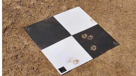
Figure 4.3: An example Ground Control Point Source: Pix4d
